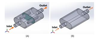
Figure 2 Muffler modeling A) baffle muffler and perforations B) muffler without baffle and perforations
