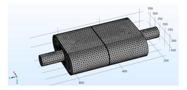
Figure 3 Mesh muffler in COMSOL software
