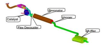
Figure 1 Schematic of an exhaust system
